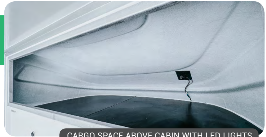
CARGO SPACE ABOVE CABIN WITH LED LIGHTS
